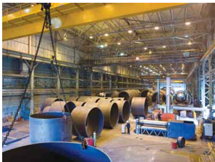
Semi-finished tower sections on motorized track mounted trolleys. Also in this area are circular and longitudinal seam submerged arc welders.
