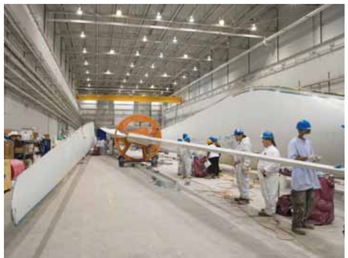
Blade finishing area where 130 foot long, 8 ton blades are sanded and repaired. Also shown are the open air cable tray systems, in floor dust collection system, and one of four bridge cranes that serve this area.
